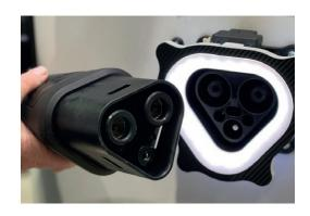
This initial release of the MegaWatt range includes air cooled couplers with a continuous rating to 350A and liquid cooled couplers to 1500A. Boost modes extending the duty-cycle rating are available for both variants. Development of the 3000A models will continue into 2024.
